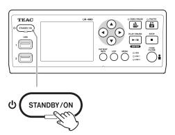
• To put the unit into standby: Press the STANDBY/ON button for about two seconds.
