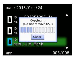
• You can cancel copying while in progress by pressing the ENTER button. 6 When the "Copy completed!" message appears, press the ENTER button to return to the list.
