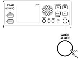
Videos and photos from before pressing the CASE CLOSE button will be stored in the same folder. The maximum number of images, including both still and video images, in one folder is 999. If this number is reached and you want to record further, press the CASE CLOSE button to end recording once. When recording is next started, a new folder will be created.
